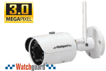
3.0 MEGAPIXEL WiFi 3.0MP Fixed Mini Bullet 3.0MP@20fps, 2.8mm (100°), 30m IR, digital WDR, 0.01lx, microSD, IP67 rated, full metal body, 12VDC VSIPW-3FBIR
