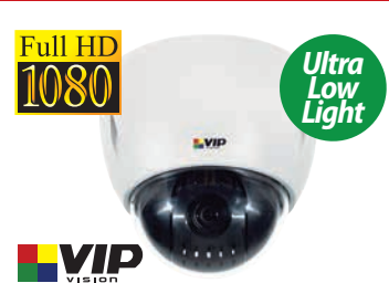
Full HD 1080 Ultra Low Light Pro 2.0MP Surface IP PTZ 2.0MP@25fps, 12x zoom 5.3~64mm lens (59° ~ 5°), endless 360° pan, 0~90° tilt, microSD, IP66, IK10 VSIP2MPPTZV3 (12 x zoom, 2.0MP)
