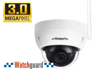
3.0 MEGAPIXEL WiFi 3.0MP Fixed Mini Dome 3.0MP@20fps, 2.8mm (100°), 30m IR, digital WDR, 0.01lx, microSD, IP67 & IK10, metal/polycarb body, 12VDC VSIPW-3VDIR
