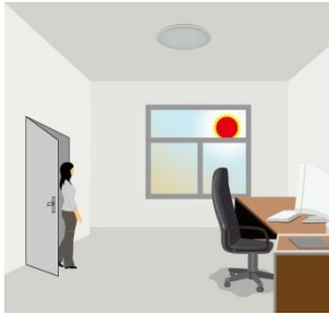
Sufficient ambient light, light does not switch on even with motion.
