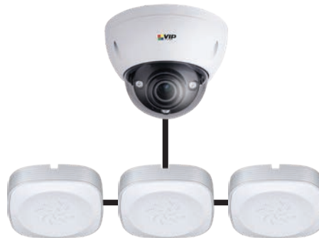
Cascade Multiple Microphones
