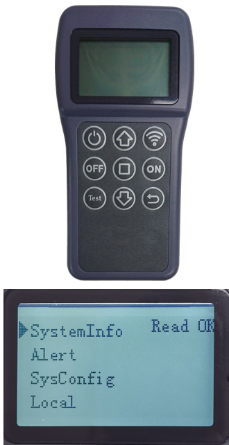
Fig. 5.1a Solar panel remote control & LCD
