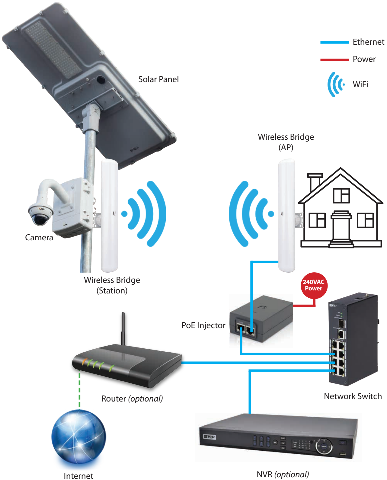
Fig. 3.1a Example WiFi Setup
